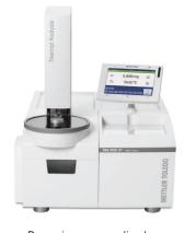
Dynamic vapor sorption by TGA Sorption Analyzer System
