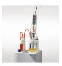
Solid samples which do not dissolve in the Karl Fischer solvent can be added to the titration vessel and ground with a Homogenizer. The Homogenizer speed is controlled by the Excellence titrator via the RS-interface and documented. This guarantees maximum security and full GLP-compliance. Special chemicals for extraction are avoided using the Homogenizer for grinding.
