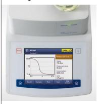
The Coulometer keeps the user informed on the cell condition and makes all tasks (e.g., sample and drift determination) available to be started with One Click<sup>®</sup>. If the expected water content is known, the optimum sample weight can be calculated. The Online Screen offers all ongoing information for the titration and direct access to all data and tasks that further accelerates the complete workflow.
