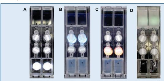
Figure 3 Guide lights underneath the Nadia cartridge chips indicate loading position of the emulsion oil (A), beads (B), cells (C) and indicate where to retrieve the emulsion (D) from after the run.
