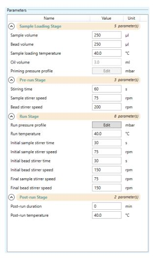
**Figure 3** Summary of editable parameters used in this agarose encapsulation application taken from the Dolomite Bio FCC software. Note that in this current version of the software (v3.22.3), parameters affecting the reservoir containing agarose are referred to as "bead".
