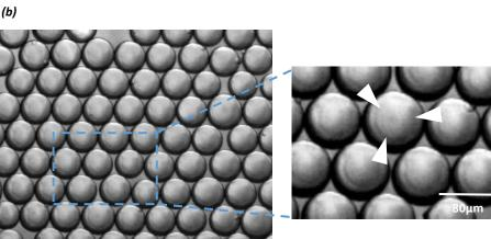
Figure 4 (a) Agarose emulsions were produced and droplet formation imaged at the Nadia Innovate chip junction The interface between cell buffer and 1.5 % agarose solution is visible (demarcated by white arrows). (b) Agarose emulsions imaged after formation show good monodispersity, with hardened agarose beads being visible inside droplets (an inlaid example of an agarose sphere within an aqueous droplet is highlighted at a higher magnification by white arrows).
