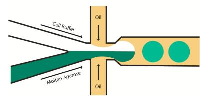
**Figure 1** Schematic of agarose droplet generation. Flow focussing allows droplets of agarose to be formed at extremely high throughput. This technique can be used to encase cells or other biological material in a spherical crosslinked scaffold once the agarose has hardened.
