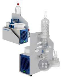
CSH System Includes chemical resistant diaphragm pump, separator, condenser, tubing
