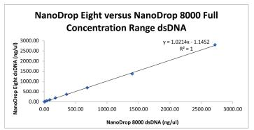
Figure 1: A linearity comparison between the NanoDrop Eight instrument versus the NanoDrop 8000 instrument across the entire concentration range for the sample dilutions. The regression line ( $R^2 = 1$ ) demonstrates that the NanoDrop Eight dsDNA concentration results were well aligned with the values obtained on the NanoDrop 8000 Spectrophotometer.
