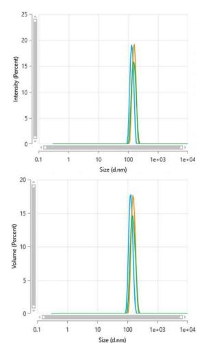
Figure 7: Malvern mastersizer (DLS) graphs of FRR 3:1:1 at a TFR of 3 mlmin-1 Intensity, number and volume distribution.
