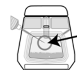
Figure 2. Needle is positioned too far inside the cassette.
