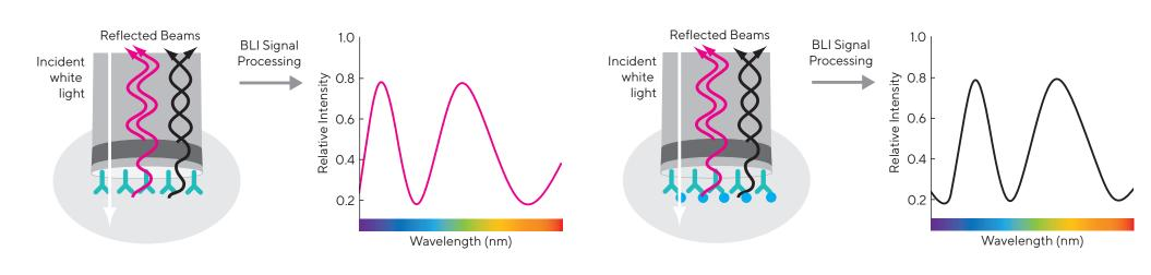
Figure 1: Principles of Bio-Layer Interferometry.
