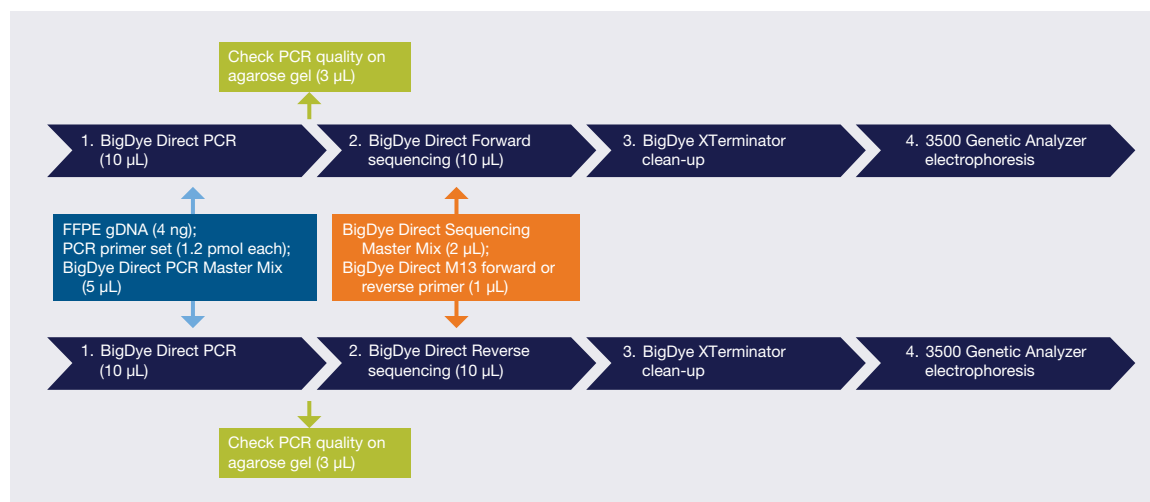
Figure 28. Workflow for BigDye Direct cycle sequencing.
