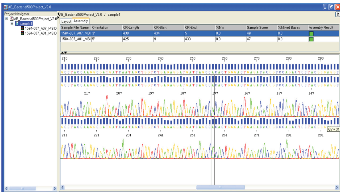
Figure 24. MicroSeq ID Analysis Software, showing the alignment of the sequences of a sample. The electropherograms of forward and reverse sequences are aligned to the consensus sequence generated by the software (at the top). The consensus sequence is compared to the validated library.
