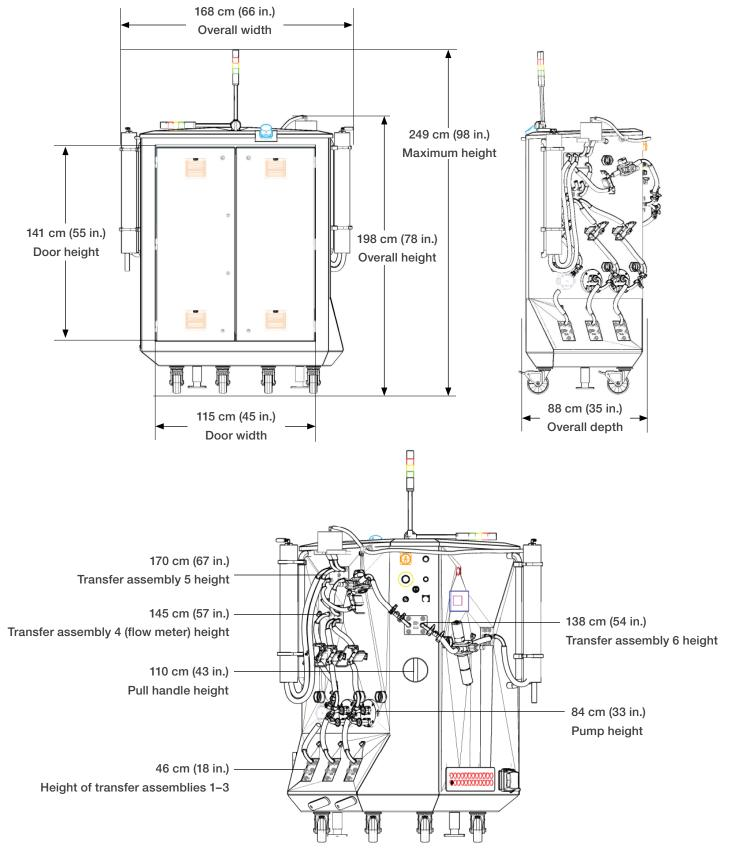
Figure 2. HyPeak Chromatography System specifications.
