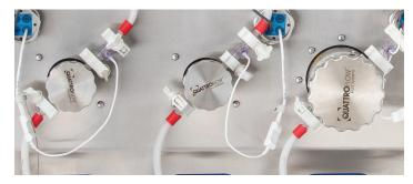
Figure 5. Three positive displacement pumps.
