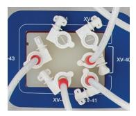
Figure 3. Fluid transfer assemblies attached to valve manifold.
