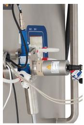
Figure 7. Post-column sensor pack with UV detector.
