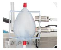
Figure 8. Bubble trap and level sensors.
