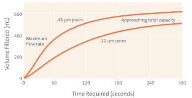
Test Conditions: Medium containing 10% fetal bovine serum was filtered using cellulose acetate membranes at 23°C and 600 mm Hg vacuum.
