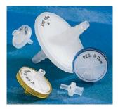
A variety of membranes are available to meet your needs: polyethersulfone (PES) – low protein binding and faster flow rates; surfactant-free cellulose acetate (SFCA) – lowest protein binding; polytetrafluorethylene (PTFE) – chemical resistance; regenerated cellulose (RC) – best choice for DMSO compatibility; nylon (NY) – hydrophilic, surfactant-free and lowest extractable.
