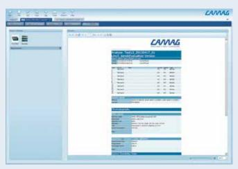
All data of the current analysis (e.g. information on the chromatogram layout, solvents used, dosage speed or application volumes) is saved by the TLC/HPTLC software in a report file.
