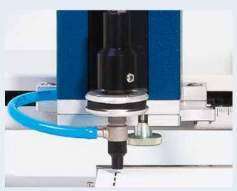
The combination of the special dosage syringe with the spray nozzle of the Linomat 5 ensures the focused spraying-on of samples on very small areas.
