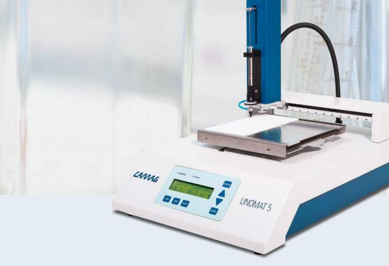
With the Linomat 5 samples are sprayed onto TLC/HPTLC plates with nitrogen or compressed air. Sample application is automatic, only changing the syringe (filling, inserting and rinsing) is manual. The Linomat is suitable for routine use.
