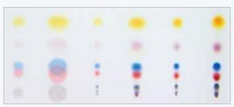
Developed plate after contact application of spots
