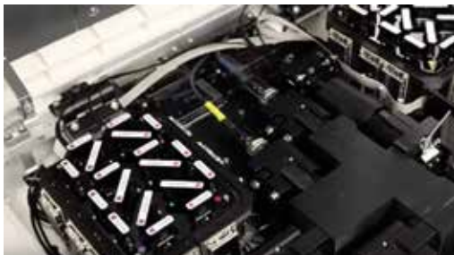
Figure 16. The optical filters in the Attune NxT Flow Cytometer are user-exchangeable, easily slotted in and out of the optical bench to maximize your capacity.
