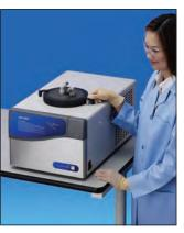
CentriVap -50 Cold Trap, which reaches -50° C (-58° F), collects moisture during evaporation to protect the vacuum pump.
