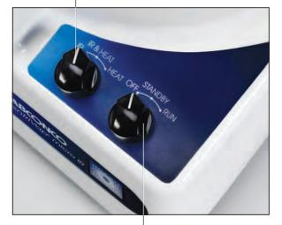
Run Mode Selector. Use to select Off, Standby (preheat) or Run mode.
