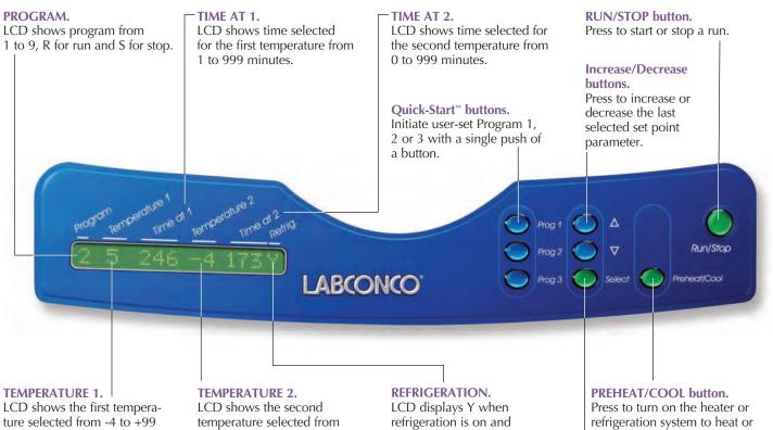
(° C) or HI (100° C). During the run, the LCD shows the actual temperature of the chamber.
