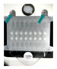
3 Follow the instructions displayed on-screen and remove gasket from chip. It can either be stored on a clean and dust-free surface or simply folded and placed behind the Nadia clamping mechanism (see below). Press "Next" to proceed.
