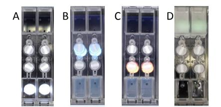
Guide lights underneath the Nadia cartridge chips indicate loading positions for the emulsion oil (A), beads (B) and cells (C), and direct the user to the emulsion (D) after the run is complete.
