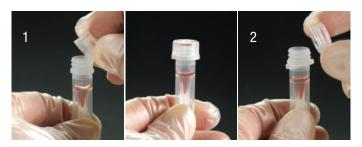
1. Screw cap until locking ring clicks over serrated tube neck.
