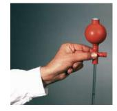
4. Blow out the pipette by pressing as the drawing indicates (point C).
