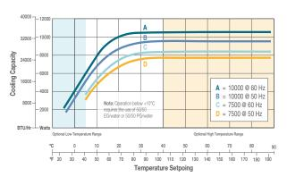
$Cooling\ capacity\ based\ on\ chillers\ with\ P2\ pumps\ with\ no\ backpressure.\ Other\ pumps\ will\ affect\ cooling\ capacity\ performance.$
