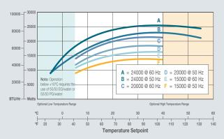
Cooling capacity based on P3 pumps set to 10 gpm.
