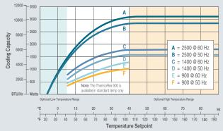
Cooling capacity based on chillers with P2 pumps with no backpressure. Other pumps will affect cooling capacity performance.
