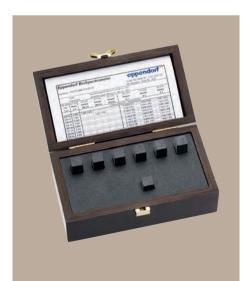
The secondary UV/Vis reference filter set is used to verify the photometric and wavelength systematic errors according to NIST (National Institute of Standards and Technology, Gaithersburg MD, USA).
