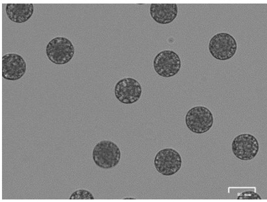
Figure 9 - 25 um PLGA dry beads containing water after DCM evaporation (bright field image). First emulsion = 5 ul/min, Aqua Phase = 50 ul/min
