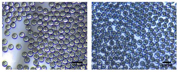
Figure 8 - 50 um PLGA beads before shrinkage with 14 um inner droplets (left) and 3 um inner droplets (right).
