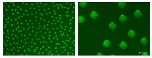
Figure 10 - 25 um PLGA dry beads containing water after DCM evaporation (fluorescent light). First emulsion = 5 ul/min, Aqua Phase = 50 ul/min
