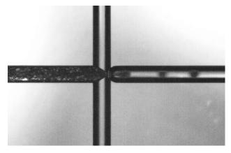
Figure 2 - Image of formation of water-in-PLGA-in-water droplets
