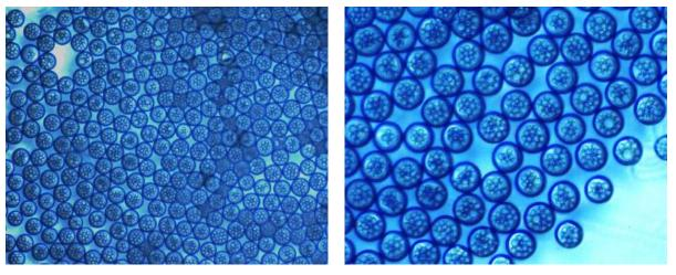
Figure 4 - Water-in-oil-in-water droplets on glass slide (bulk)
