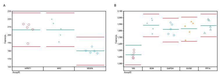
**Figure 5. QuantStudio**<sup>®</sup> **3D Digital PCR System precision.** Five independent technical replicates were generated across an 8-assay panel of TaqMan<sup>®</sup> Gene Expression Assays. All measurements were within ±10% (red lines) of the respective means (green lines). **(A)** Results for low expressors—HPRT1, MYC, and VEGFA. **(B)** Results for higher expressors—18S, B2M, GAPDH, GUSB, and PPIA.
