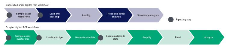
**Figure 2. Chip-based digital PCR workflow: more streamlined and secure than droplet-based workflow.** The QuantStudio<sup>®</sup> 3D chip-based digital PCR workflow involves minimal pipetting steps and a sealed system (once the chip is closed). In comparison, a droplet-based approach requires more pipetting steps as well as multiple transfer steps, which expose the sample to potential contamination.
