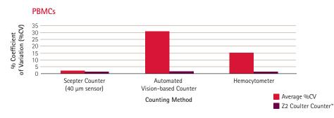
The Scepter 2.0 cell counter counts PBMCs with greater precision than other counting methods, as reflected by low coefficients of variation. %CVs were calculated using average cell counts of four replicate samples.
