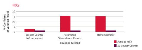
The Scepter 2.0 cell counter counts RBCs with greater precision than other counting methods, as reflected by low coefficients of variation. %CVs were calculated using average cell counts of four replicate samples.
