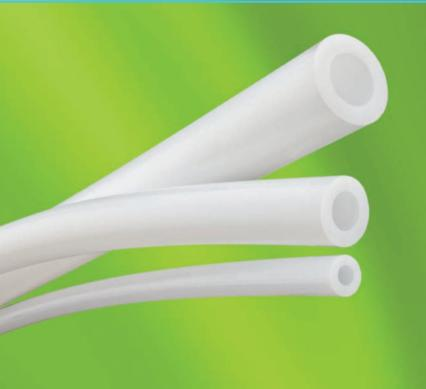
PTFE-reinforced silicone tubing which provides long term performance with repeatable accuracy, vital in pharmaceuticals and other high technology industries. Suitable for pressures up to 7 bar (100 psi), GORE STA-PURE PCS provides the longest available tube life with virtually no spallation.
