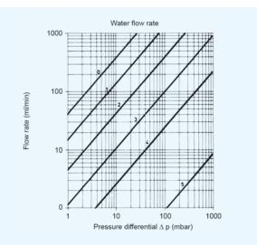
Water flow rate through filter discs of various porosities as a function of pressure differential. For filter discs with Ø 30 mm
