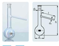
Uniform wall thickness distribution makes these flasks ideal for heating applications and distillations. DURAN® Engler Distilling Flasks comply with the requirements of ASTM D86 and DIN EN ISO 3405 for the atmospheric distillation of petroleum products.
