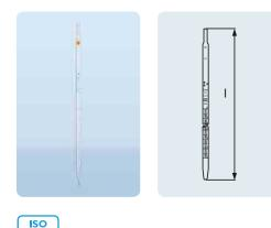
Numbering: zero at bottom. Calibration is based on the poured out volume ("Ex") at a + 20 °C reference temperature. Due to the scale, variable volumes can be held and then dispensed in the same or differing increments.
