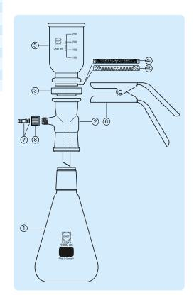
Typical applications: Coarse and fine filtration, filtration of HPLC media, residue analysis.
