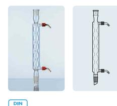
The bulb condenser has a greater cooling surface than the liebig condenser and thus higher cooling capacity.
