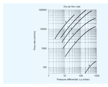
Air flow rate through filter discs of various porosities as a function of pressure differential. For filter discs with Ø 30 mm
