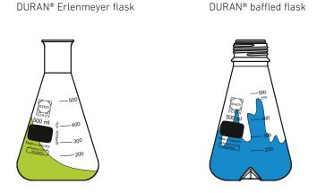
The movement causes a liquid sickle to form when using DURAN® Erlenmever flasks on a vibrator. The DURAN® baffled flask with four baffles on the bottom disrupts the laminar flow and produces a turbulent flow. The surface area of the liquid and the gas-exchange area are increased, thereby increasing the oxygen intake.
