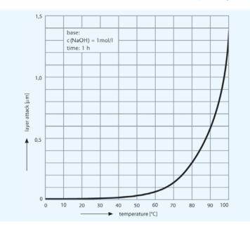
Alkali attack on DURAN® as a function of temperature (°C)
