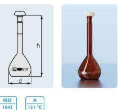
Calibration is based on the poured in volume ("In") at a + 20 °C reference temperature. The volume content tolerances conform to accuracy class A, the accuracy limits of the German weights and measures regulations and DIN and ISO specifications.
