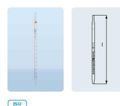
Numbering from the top down. Calibration is based on the poured out volume ("Ex") at a + 20 °C reference temperature. Due to the scale, variable volumes can be held and then dispensed in the same or differing increments.
