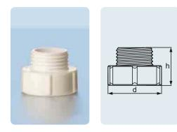
The re-usable adaptor (GL 45 external / GL 56 internal) allows the use of the DURAN® *TILT* bottle with 45 mm filtation units for the filter sterilisation of cell culture media. Manufactured from inert PTFE; can be autoclaved and depyrogenised at 300 °C.
