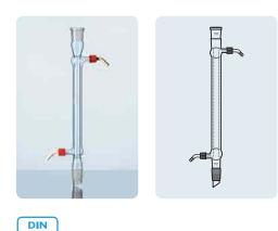
Relatively small heat exchange surface and thus relatively low cooling capacity.
