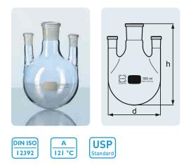
Thanks to the uniform wall thickness, round bottom flasks are ideal as heating vessels. The geometry permits very uniform heating. Depending upon the application, accessories, columns, thermometers, dropping funnels, boiling capillaries, etc. can be fitted.
