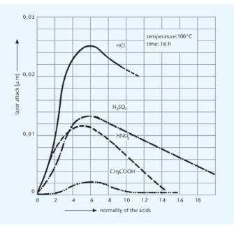
Acid attack on DURAN<sup>®</sup> as a function of acid concentration
