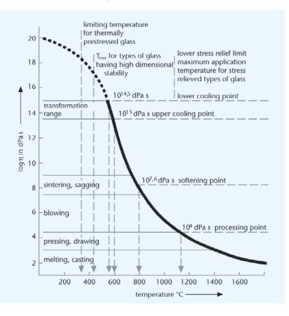
Normal temperature dependence/viscosity curve of, for example, DURAN®; viscosity ranges of important processing techniques, position of fixed points of viscosity and various limiting temperatures.
