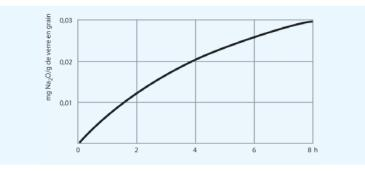
Hydrolytic attack on DURAN® as a function of time (h)
