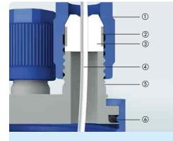
Schematic diagram of GL 45 connection system
