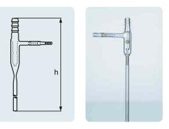
Throughput: 400 l/h at 3.5 bar water pressure und 12  $^{\circ}\mathrm{C}$  water temperature.
