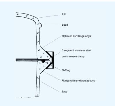
Beaded lid for safer handling of the reaction vessel
