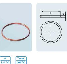
Accessories for flat flange vessels, comprising an elastic, silicone core with seamless FEP coating that encloses the ring. The combination of these high-quality materials achieves good elasticity in conjunction with outstanding chemical resistance.
