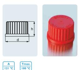
Suitable for PBT screw caps and tamper-evident screw caps. Heat resistance: 130 °C (vapour) and 200 °C (dry heat). Good chemical resistance due to PTFE coating. Silicon is peroxidically cured.
