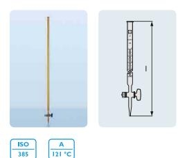
With main graduations as circular divisions. Calibration is based on the poured out volume ("Ex") at a + 20 °C reference temperature. Volume content tolerances conform to DIN.
