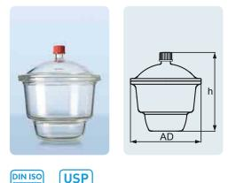
Typical applications: drying of moist samples and storage of moisture-sensitive substances.
