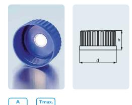
For GLS 80® thread. Ideal for autoclaving processes because the 0.2 micron ePTFE membrane permits pressure equalisation and screw tight sealing. Hence the risk of contamination is greatly reduced. Ingress of liquids or solids is prevented and the bottle contents remain sterile.
