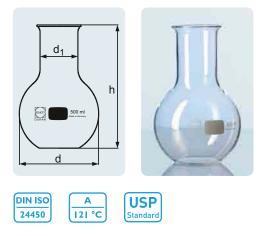
Uniform wall thickness distribution makes these flasks ideal for heating applications and distillations. DURAN<sup>®</sup> Engler Distilling Flasks comply with the requirements of ASTM D86 and DIN EN ISO 3405 for the atmospheric distillation of petroleum products.
