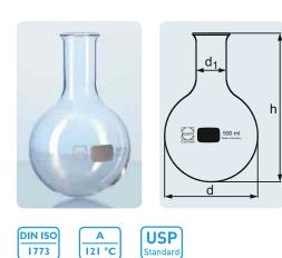
Uniform wall thickness distribution makes these flasks ideal for heating applications. The geometry permits very uniform heating. Flasks with a neck diameter of  $65\,\text{mm}$  or more have a reinforced rim.
