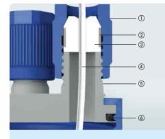
Schematic diagram of GLS 80<sup>®</sup> connection system
