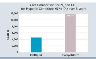
Representative comparison of cost (setpoints 5% CO<sub>2</sub> / 5% O<sub>2</sub>, 37°C, 3 door openings per day at 5 days a week, 4-segmented inner doors)
