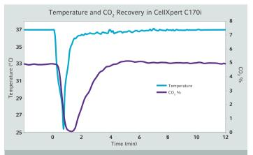
Temperature and CO<sub>2</sub>-recovery following 30 s door-opening. Notice the typical regulative oscillations before the initial value is reached.
